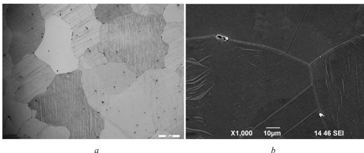
**Fig. 1.** Structure of magnesium alloy Mg-1%Zn-0.2%Ca in the initial state:
