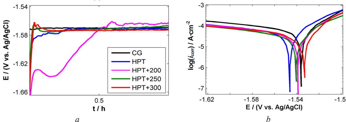
**Fig. 4.** Electrochemical test results for Mg-1%Zn-0.2%Ca in Ringer solution:
