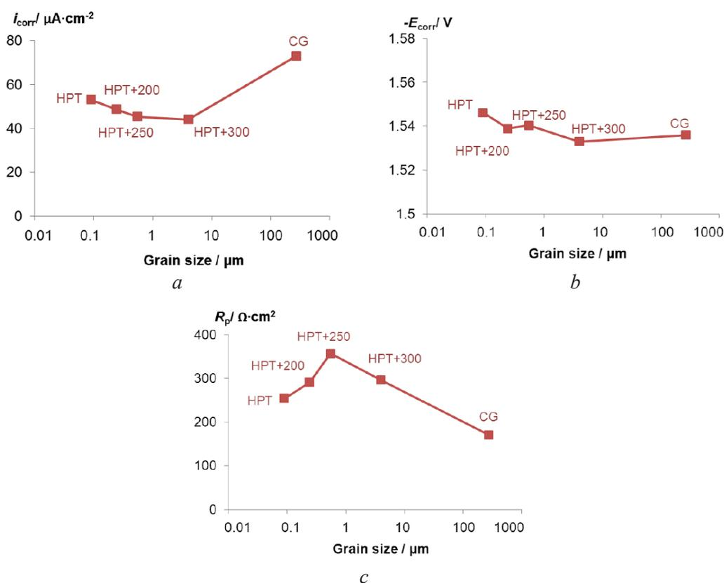
**Fig. 5.** Electrochemical test results for Mg-1%Zn-0.2%Ca in Ringer solution: *a* – corrosion current density  $i_{\text{corr}}$ ; *b* – corrosion potential  $E_{\text{corr}}$ ; *c* – polarization resistance  $R_p$
